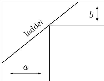
**Answer:** (1)  $L = \sqrt{a^2 + x^2} + \sqrt{b^2 + y^2}$  and  $x/a = b/y$ , so  $L = (1 + b/x)\sqrt{a^2 + x^2}$ .  $L' = 0$  for  $x = (a^2b)^{1/3}$ . Then  $L = (a^{2/3} + b^{2/3})^{3/2}$ .
